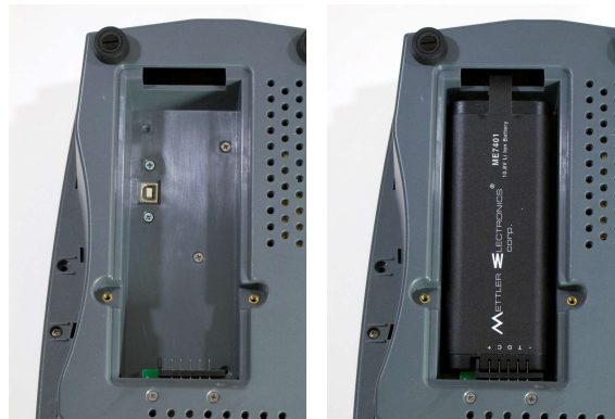
Figure 3.2— Sys*Stim 240, Bottom View— Installing the battery
